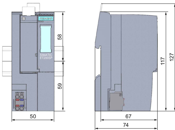
Figure A-1 Dimension drawing of the IM 155-6 PN ST interface module (front and side view)
